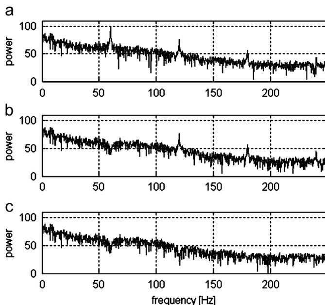
Fig. 6. Power spectrum of the: (a) acquired EEG signal; (b) EEG signal processed by the conventional canceller [10]; (c) EEG signal processed by the proposed algorithm.
