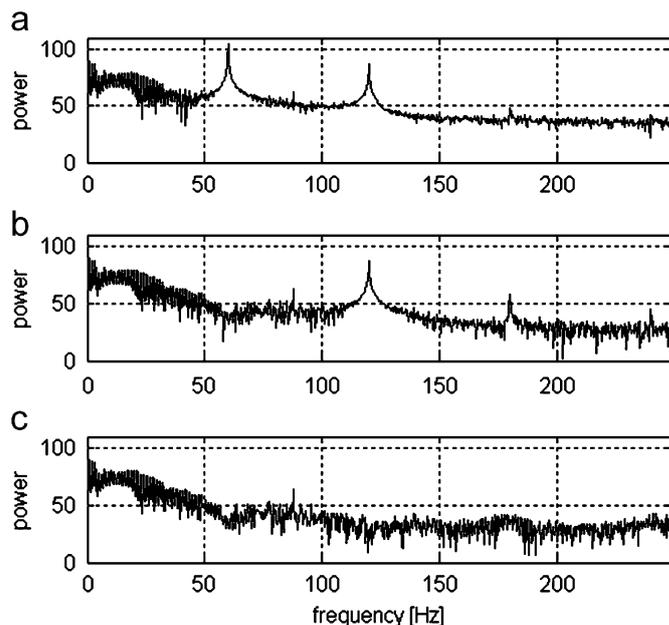
Fig. 5. Power spectrum of the: (a) acquired ECG signal; (b) ECG signal processed by the conventional canceller [10]; (c) ECG signal processed by the proposed algorithm.
