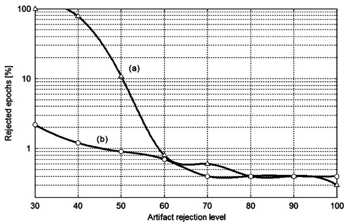
Fig. 8. Rejected epochs in the most contaminated MLAEP of a patient under surgery: (a) conventional canceller and (b) proposed algorithm.
