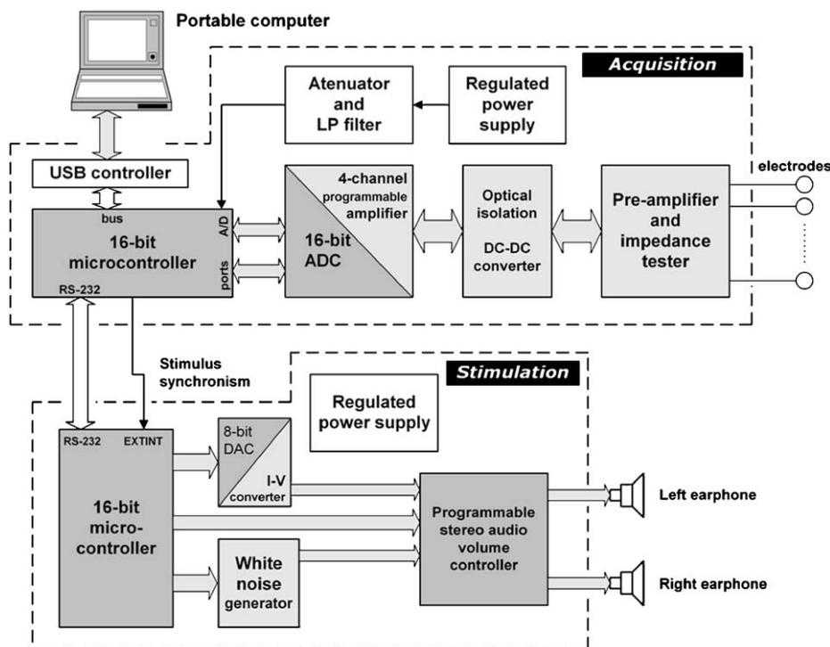
Fig. 3. Block diagram of the acquisition hardware [15].
