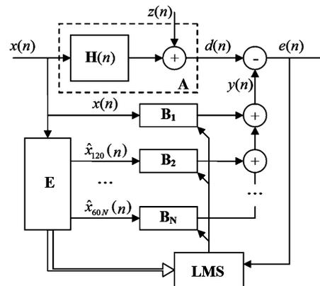
Fig. 2. Block diagram of the proposed adaptive noise canceller (60 Hz notation).
