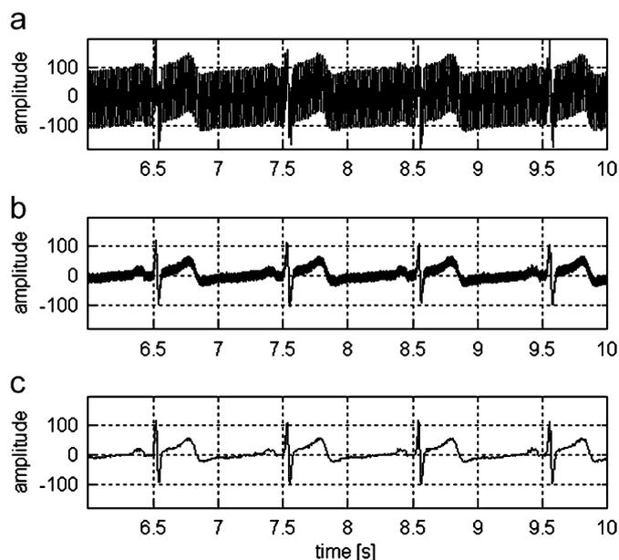
Fig. 4. Time evolution of the: (a) acquired ECG signal; (b) ECG signal processed by the conventional canceller [10]; (c) ECG signal processed by the proposed algorithm.
