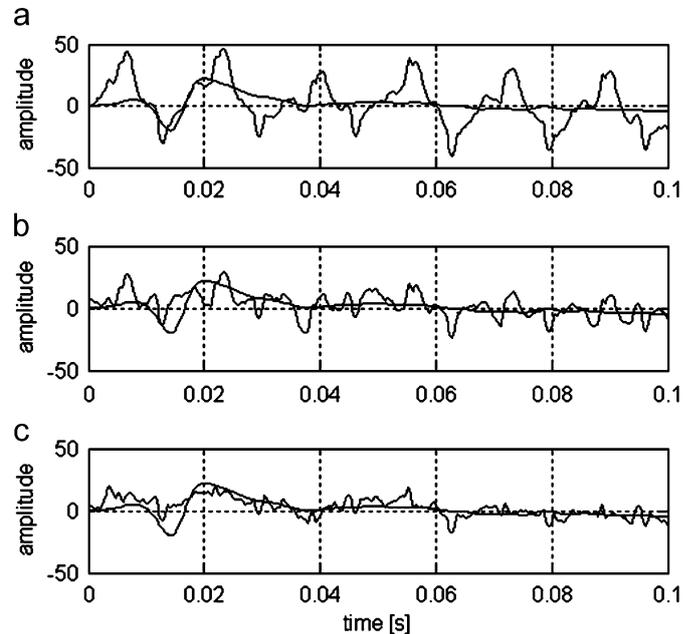
Fig. 10. Time evolution of the: (a) EEG signal; (b) EEG signal processed by the conventional canceller; (c) EEG signal processed by the proposed algorithm. A scaled version of the averaged MLAEP (1000 epochs, scale factor of 7) is synchronously superimposed with all plots (smoothed line).
