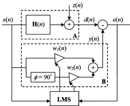
Fig. 1. Block diagram of the Widrow's conventional adaptive noise canceller [10].
