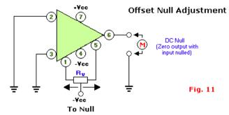
Note: Both inputs grounded as shown above implies that Vin is zero and that each input has a DC resistance path to ground. The actual resistance depends on the application.
